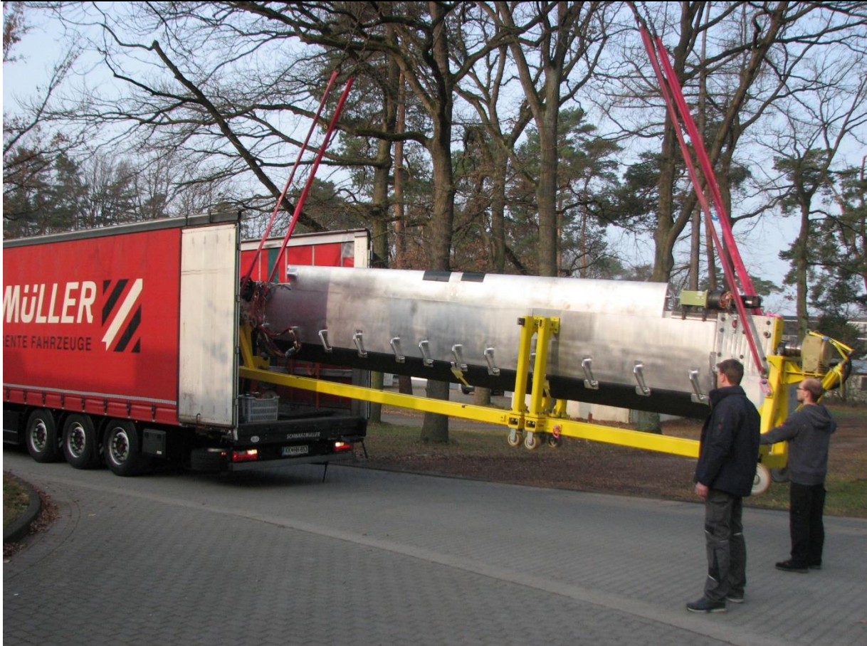
Figure 23: loading the assembled DLR-F15LS model into the truck for transport to DNW-LLF
