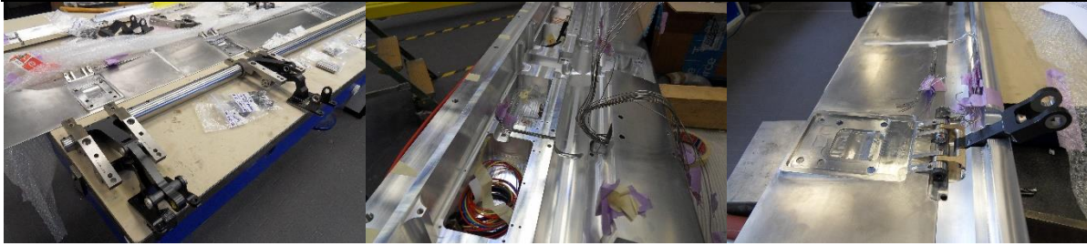
Figure 21: impressions of pre-assembly and instrumentation of the DLR-F15LS model parts: (left) drive train & kinematics; (middle) cabling and pressure tube installation in leading edge; (right) pre-assembly of Krueger flap and pressure tube installation
