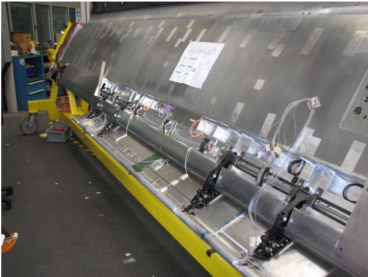
Figure 22: assembled DLR-F15LS model with Krueger mounted during instrumentation installation
