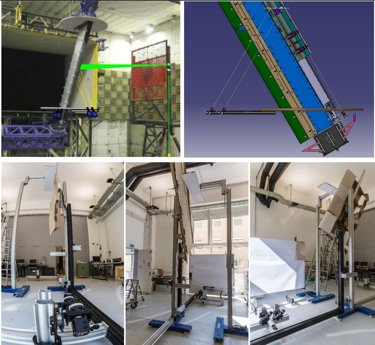
Figure 29: planned PIV installation in DNW-LLF and digital mock-up (DMU) (top-row) and corresponding laboratory mock-up (bottom-row) to check visibility, camera angles and optics.
