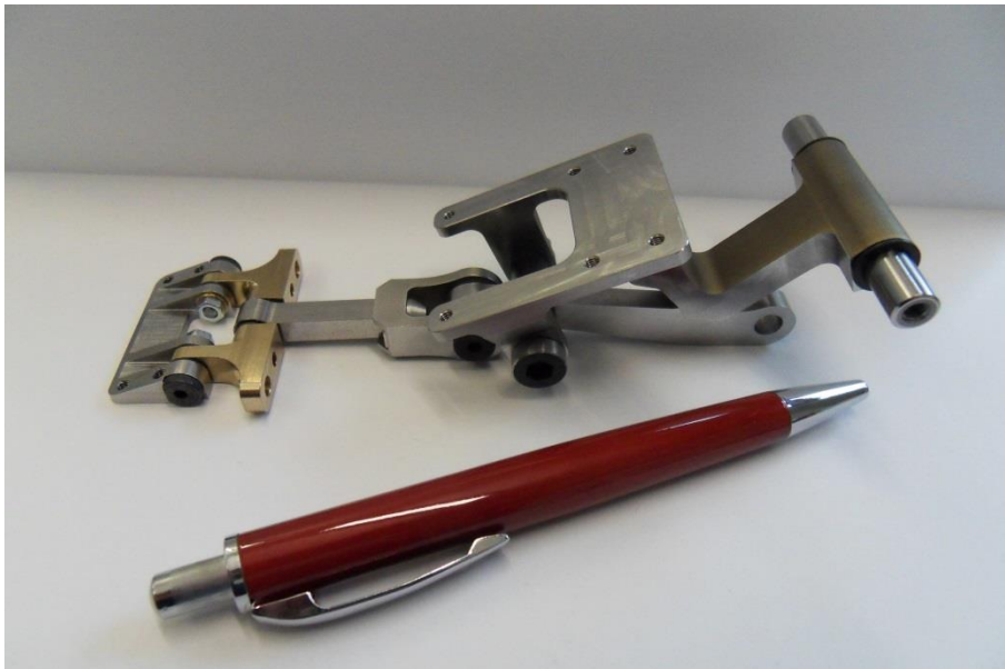
Figure 16: manufactured Krueger kinematics for the DLR-F15 model
